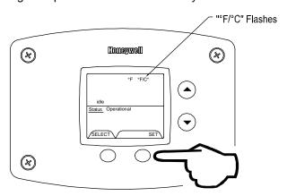
Step 3a: Press "Temperature Up" button to change temperature format to °C
